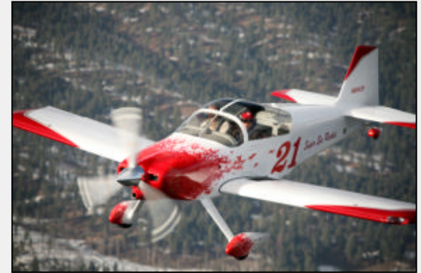
Carl Brownd's RV-6, the Super Six Rocket, is a rare taildragger with side-by-side seating.
