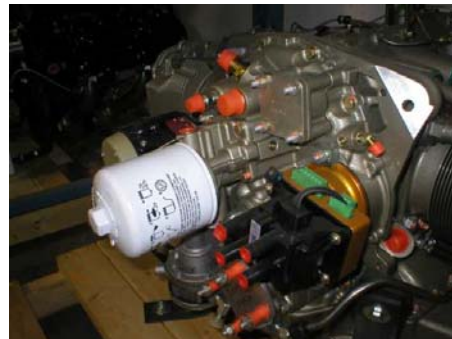
Straight spin-on adapter, oil filter, gasket and mounting stud - $180.00
